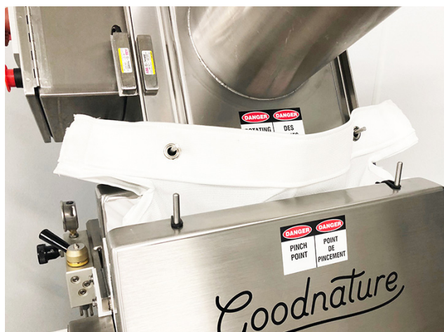
Fig 3.1: Press bag in grinding position
