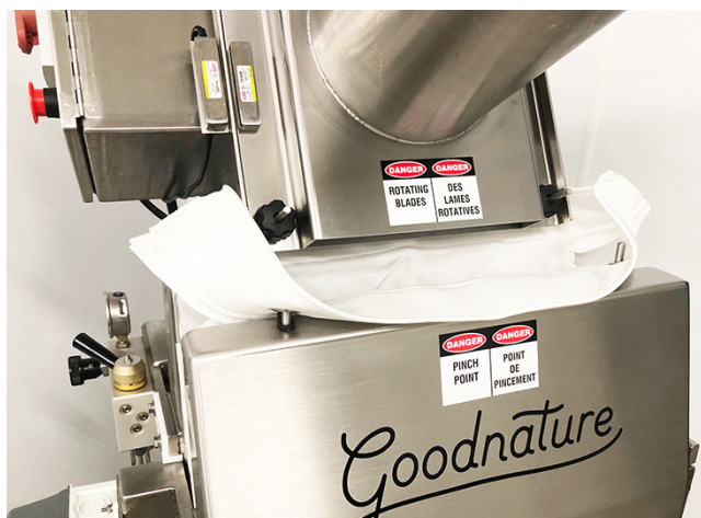
Fig 3.2: Press bag in pressing position
